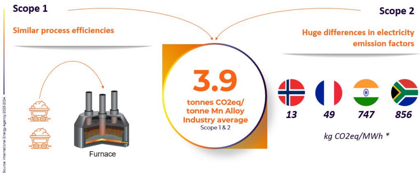
Figure 4. Illustration explaining why manganese alloys Scope 2 is very different among the producers
