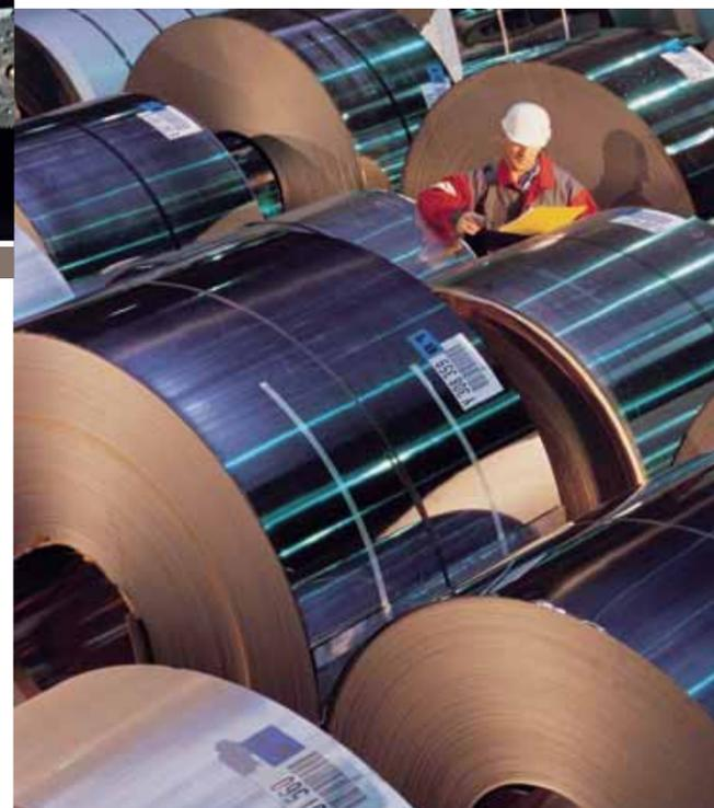
Containing 8-12% nickel, stainless steel is by far the largest outlet for the nickel industry.
