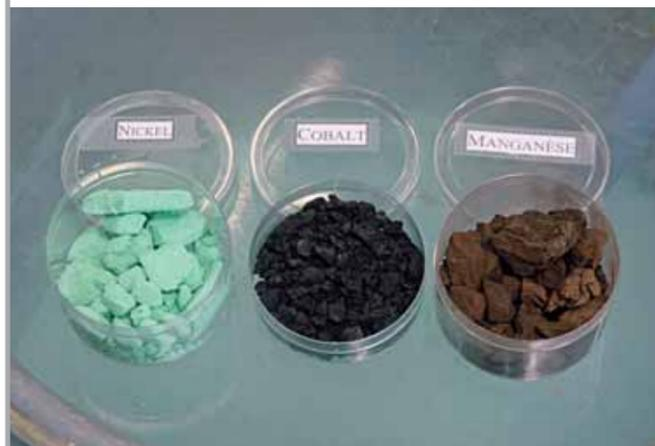
Products resulting from the hydrometallurgical method for nickel ore beneficiation, processed in Group plants or elsewhere.
