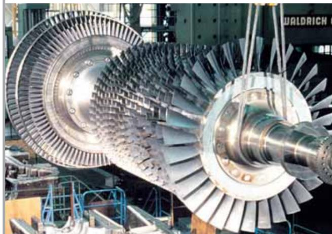
Aubert & Duval closed die-forges parts for power turbines.
