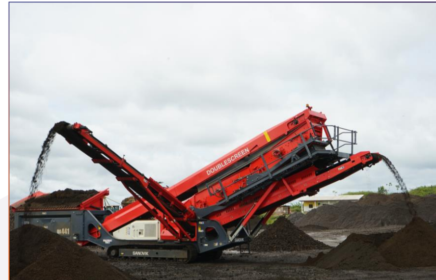
Manganese ore dry processing in Gabon: crushing and screening equipment
